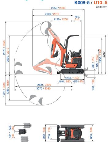
\* Working ranges are with Kubota original bucket, without quick coupler. \*Specifications are subject to change without notice for purpose of improvement.
